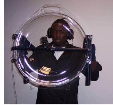
Figure 3. A commercial parabolic dish microphone used to improve hearing.
